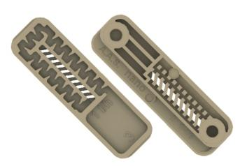
Specially designed labyrinth creates turbulent flow, thus preventing clogging of the emitter
