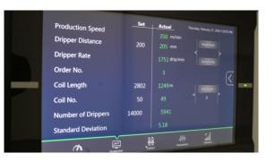
The HMI provides detailed statistics, data and graphs of the production line operation, along with a complete set of the production output data. Those functions transform the HMI to a powerful decision-making tool for production planning, cost analyzing, efficiency and effectiveness increasing and so on. Moreover, it is a user-friendly ad hoc monitoring of the production.
