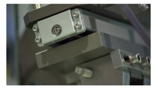
We have designed and developed a unique air vacuum system, which removes and stores the part of the pipe that has been cut during the drilling process. This leads to a totally clean space around the drilling unit, without any cutting chips.
