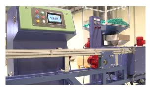
the feeder. This combination ensures the perfect balance between the pre-feeder and the inserting unit. The feeder acts as a balance connection point of the overall feeding unit, between the emitter storage which is the pre-feeder and emitter destination, the inserting unit.
