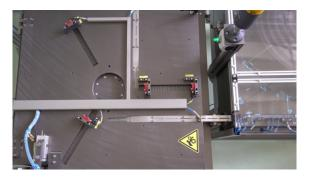
Sensing system which is able to provide several acoustic and visual alarms depending on the preset settings. This enhances the seamless operation of the production line and secures the optimum production capability.
