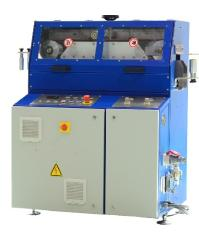
The great built quality of our caterpillar ensures its durability and the high performance of the unit. It is equipped with poly-V belts which guarantees a perfectly aligned movement of the belt and dripline. By designing it from scratch and carefully selecting special materials for our caterpillar, we have managed to develop a noiseless
