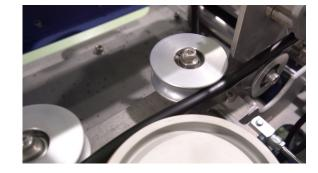
functions of a drip irrigation production line. This is why we have put a lot of effort in designing and developing the most advanced drilling unit in the industry. Capable of coping with the drilling demand of a high-speed production, of 120 meters per minute. The operating capacity of our driller is up to 500 emitters per minute, making it the fastest drilling unit in this segment of the industry.
