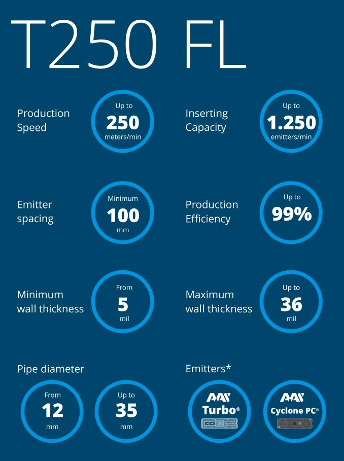
\* Turbo and Cyclone PC equivalent emitters can be used with T250 FL production line.
